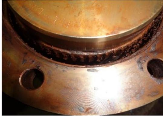
Gambar 1. Keausan *Gear Coupling Ballast Pump*
