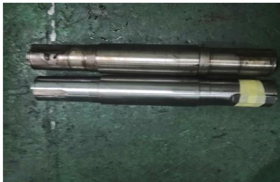
Gambar 2. *Shaft Gear Coupling Ballast Pump*
