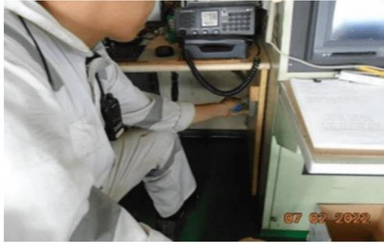
Gambar 14. Tombol *Ship Security Alert System* (SSAS) kapal MT. B Ocean
